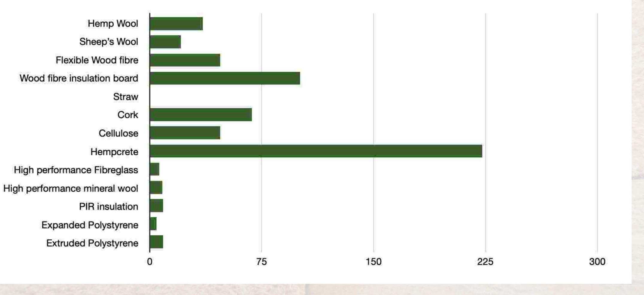
Energy Storage per m2 with 5 degree temperature change (kJ/m2)
